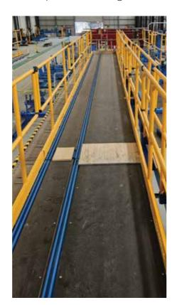
With dimensions spanning 20 meters in length, 1 meter in width, and 2.4 meters in height, the platform is engineered to meet the specific requirements of Alstom's tram production.
